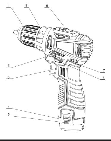
2. LED light 3. on/off switch 4. Battery pack 5. Battery lock knob 6. steering lever
